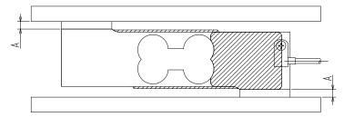
When the fitting, the load cell must be spaced apart from the loading plate and the base plate at a distance of "A" ("A" is shown in above figure). A slight deformation of load cell has been occurred under loading, which may cause contact between the silicon-coat and plates. "A" is depend on the product and a usage, we recommend the distance of 3mm to 5mm.
