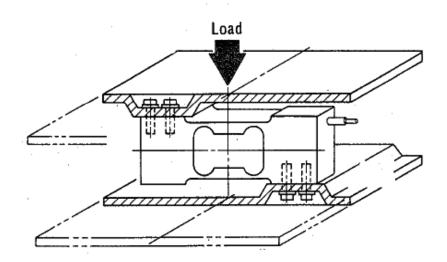
when used for a balance, install it in such a way the center of load cell is in accord with that of the loading plate. Check the size of loading plate, referring to the catalogue or specification.
